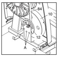
elliptical exerciser until the Belt (84) is tight, and then tighten the three screws.
